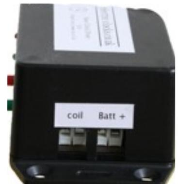
It is **ESSENTIAL** that the battery connections are made the correct way around
